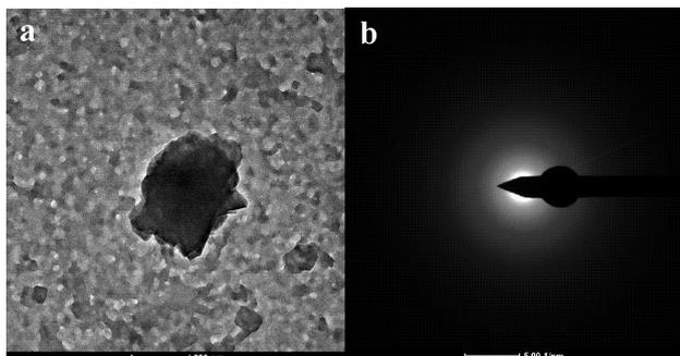
**Figure 11.** Panel (a) shows the TEM image and (b) SAED pattern of an O-, S-, and Co-containing particle obtained from an ascending gas flow in the soil from the Qingmingshan Cu–Ni sulfide deposit, Guangxi province.
