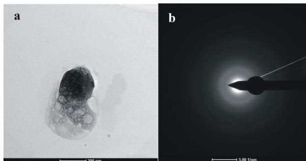
**Figure 5.** Panel (a) shows the TEM image and (b) SAED pattern of an S-, O-, K-, Na-, and Pb-containing particle obtained from an ascending gas flow above the soil over the Dongshengmiao deposit.
