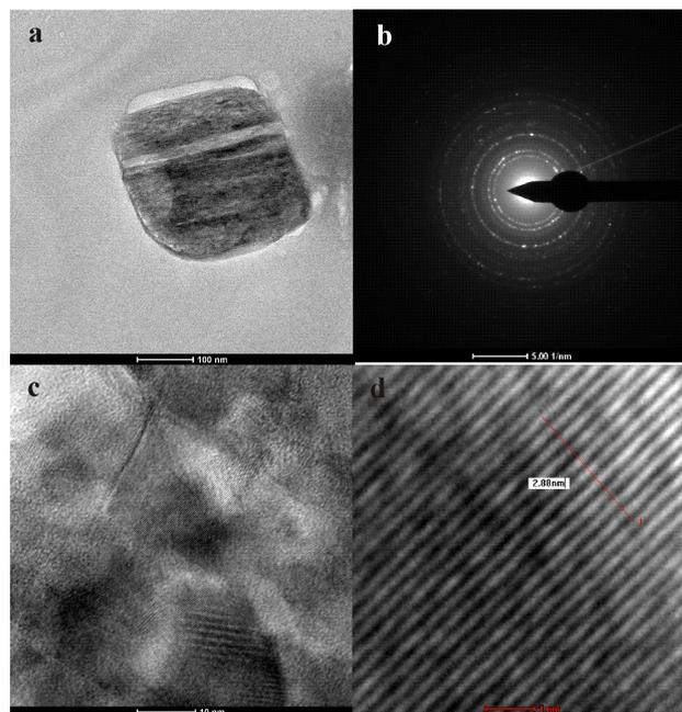
**Figure 8.** Panel (a) shows the TEM image, (b) SAED pattern, and (c), (d) HRTEM image of an O-, S-, Ca-, and Mg-containing particle obtained from an ascending gas flow in the soil over Dongshengmiao deposit.
