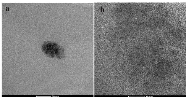
**Figure 6.** Panel (a) shows the TEM image and (b) HRTEM image of an O-, Si-, S-, and Cu-containing particle aggregation obtained from an ascending gas flow above the soil over the Dongshengmiao deposit.
