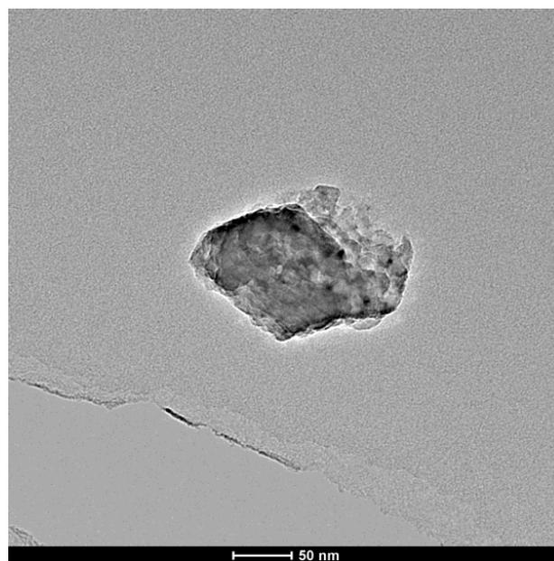
**Figure 16.** TEM image of an O-, S-, Fe-, Co-, and Ca-containing particle from a deep-seated fault gouge in the Dongshengmiao deposit.
