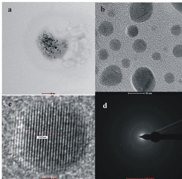
**Figure 13.** Panel (a) shows the TEM image, (b), (c) HRTEM images, and (d) SAED pattern of an O-, S-, and K-containing particle aggregation sampled using a PVC pipe in a fault near a concealed ore body of the Dongshengmiao deposit.
