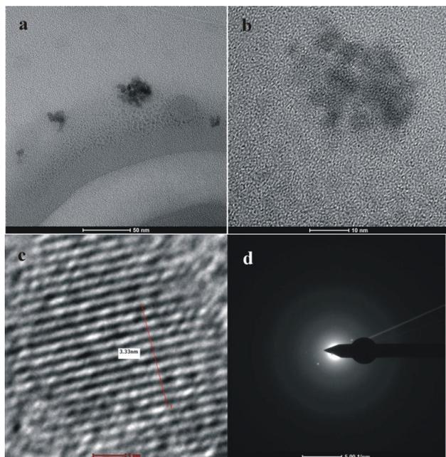
**Figure 2.** Panel (a) shows the TEM image, (b), (c) high-resolution (HRTEM) images, and (d) selected area electron diffraction (SAED) pattern of an S-, O-, Hg-containing particle aggregation obtained from an ascending gas flow above the soil over the Dongshengmiao deposit.
