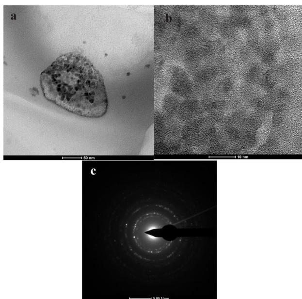
**Figure 7.** Panel (a) shows the TEM image, (b) HRTEM image, and (c) SAED pattern of an O-, S-, K-, and Pb-containing particle aggregation obtained from an ascending gas flow above the soil over the Dongshengmiao deposit.
