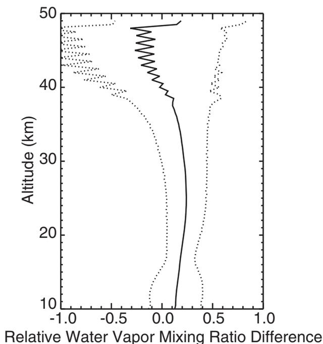
**Fig. 13.** The mean relative difference between SAGE III Version 4 water vapor mixing ratio profile with Version 3. The dotted lines show the range defined by 1 standard deviation ( $\pm 1-\sigma$ ).
