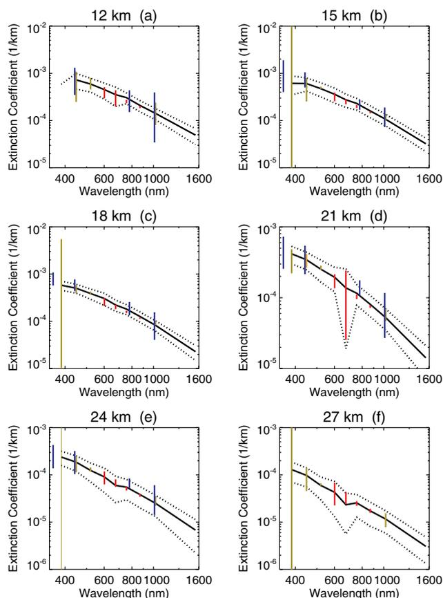
**Fig. 5.** Mean aerosol extinction coefficient spectra from SAGE III as solid line with 1- $\sigma$  standard deviation shown as a dotted line with matched SAGE II (green), POAM III (blue), and values interpolated from SAGE III values at 449, 520, and 1020 nm using an Angstrom model (red) as vertical lines spanning  $\pm 1\text{-}\sigma$ . Data is shown at 12 (a), 15 (b), 18 (c), 21 (d), 24 (e), and 27 km (f).
