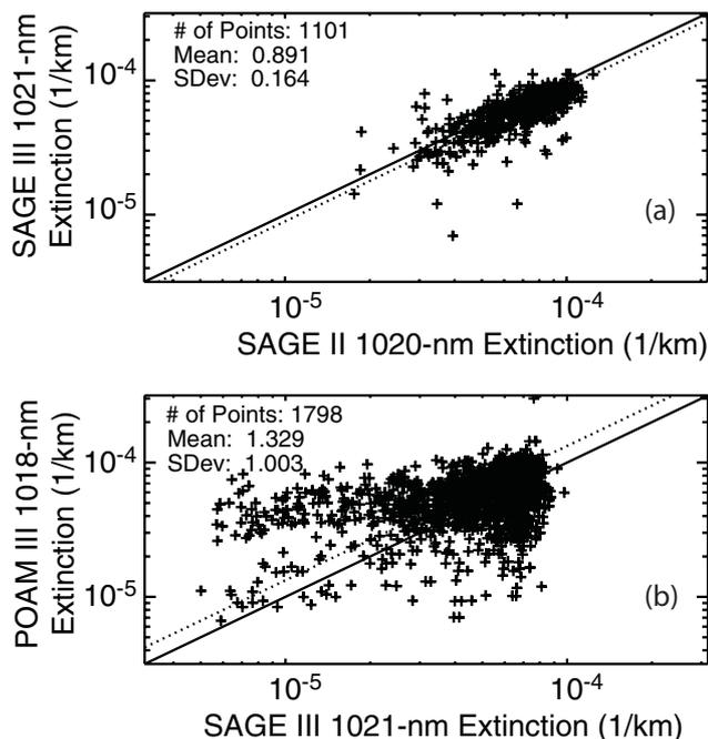
**Fig. 2.** Comparison of coincident pairs at 20 km for SAGE III version 4 1020-nm aerosol extinction coefficients with data from SAGE II (a) and POAM III (b). For frame (a), a total of 1101 matched points were used with a mean of 0.891 and a standard deviation of 0.164. For frame (b), the number of points used is 1798 with a mean of 1.329 with a standard deviation of 1.003.
