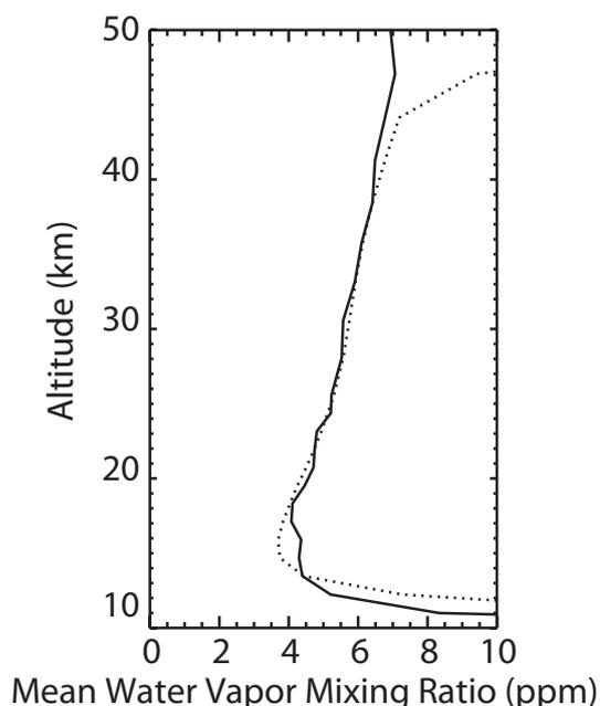
**Fig. 16.** Mean SAGE III (dotted) and MLS (solid) water vapor mixing ratio profiles for  $\sim 8000$  coincident events from mid-2004 through 2005.
