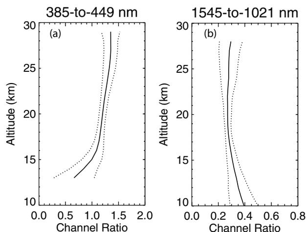
**Fig. 8.** Profiles of the average extinction coefficient ratios at 385-to-449 nm (a) and 1545-to-1021 nm (b) for all SAGE III events. The mean is shown as a solid line and the range defined by  $\pm 1\sigma$  are shown as dotted lines.
