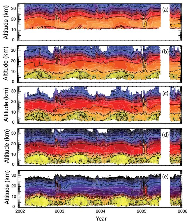
**Fig. 1.** SAGE III aerosol extinction coefficient at 385 (a), 520 (b), 676 (c), 869 (d), and 1545 nm (e) from February 2002 to December 2005 in bins of 0.02 years by 0.5 km requiring at least 5 data points per bin. Isoleths of extinction coefficient (1/km) are given every 0.5 cycles of log base 10; color contours are given every 0.1 cycles of log base 10. The lowest values of extinction coefficient are shown as dark blue and the largest values are shown as yellow.
