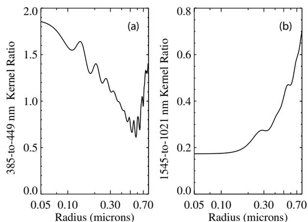
**Fig. 9.** The ratio of Mie extinction coefficient kernels at 385-to-449 nm (a) and 1545-to-1021 nm (b) for 25%  $\text{H}_2\text{SO}_4$ /75%  $\text{H}_2\text{O}$  aerosol at stratospheric temperatures.
