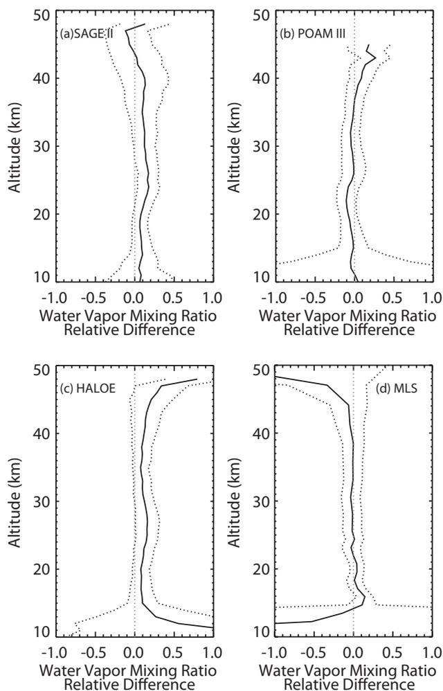
**Fig. 15.** Profile of the mean difference (other instrument/SAGE III) between SAGE III version 4 water vapor mixing ratio with SAGE II (a), POAM III (b), HALOE (c), and MLS (d). The dotted lines show the range defined by 1 standard deviation ( $\pm 1\text{-}\sigma$ ).
