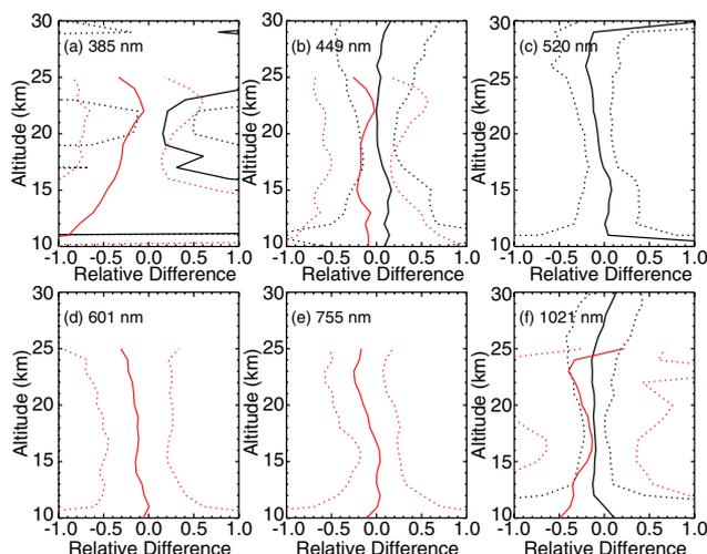
**Fig. 4.** Profile of the mean difference between comparisons of SAGE III version 4 aerosol extinction coefficient at 385 nm (a), 449 nm (b), 520 nm (c), 601 nm (d), 755 nm (e), and 1021 nm (f) with spectrally close channels from SAGE II (black) and POAM III (red) as solid lines. The dotted lines show the range defined by 1 standard deviation ( $\pm 1\sigma$ ).
