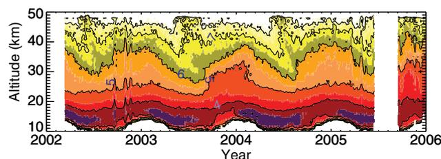
**Fig. 14.** SAGE III water vapor mixing ratio from February 2002 to December 2005 in bins of 1 week by 0.5 km requiring at least 5 data points per bin. Isoleths of mixing ratio are given every 1.0 ppm; color contours are given every 0.5 ppm. The lowest water vapor mixing ratios are shown as purple and the largest values are shown as yellow.
