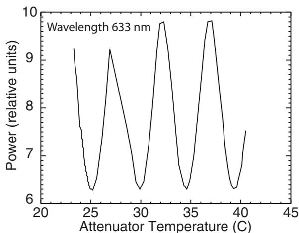
**Fig. 10.** The power throughput of a 633-nm HeNe laser through a sample of the SAGE III solar attenuator as a function of temperature.
