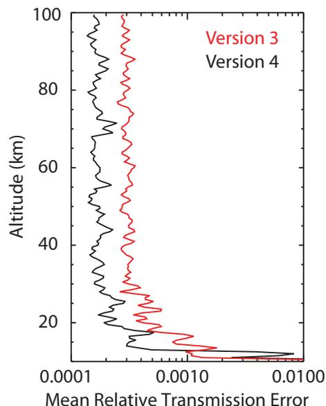
**Fig. 12.** Mean transmission error for the 28 channels in SAGE III water vapor band as a function of altitude for Version 4 (black) and Version 3 (red).
