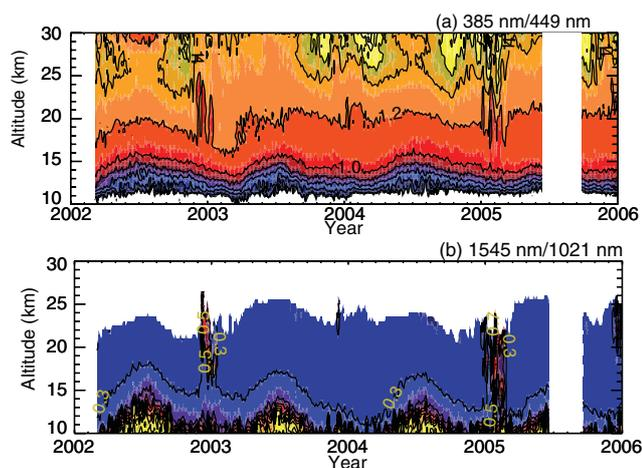
**Fig. 7.** SAGE III aerosol extinction coefficient ratio for 385-to-449 nm (a), and 1545-to-1021 nm (b) from February 2002 to December 2005 in bins of 0.02 years by 0.5 km requiring at least 5 data points per bin. Isoleths of extinction ratio are given every 0.2; color contours are given every 0.1. The smallest values of extinction ratio are shown as dark blue and the largest values as yellow.
