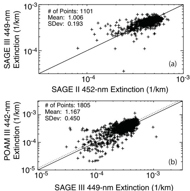
**Fig. 3.** Comparison of coincident pairs at 20 km for SAGE III Version 4 449-nm aerosol extinction coefficients with data from SAGE II at 452 nm (a) and POAM III at 442 nm (b). For frame (a), 1101 matched points were used with a mean of 1.006 and a standard deviation of 0.193. For frame (b), 1805 points were used with a mean of 1.167 and a standard deviation of 0.450.
